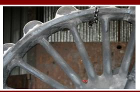
It would be two days before the fierce liquid heat would cool to a tarnished silver, and the mould would be cracked open to reveal the wheel within. Then the work started. The pouring risers had to be machined off and the wheel shot-blasted clean until it was a gleaming, gunmetal grey. Then it was whisked away for x-raying and heat treatment, whilst work began on the remaining five driving wheels.
