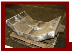
The nearly completed bogie bolster is seen at the Boro Foundry on 15<sup>th</sup> September 2010. Further machining was due to take place before being delivered to Llangollen for fitting on 'The Unknown Warrior'. Photo by Bob Sweet.
