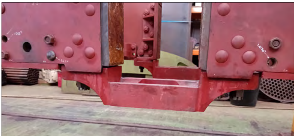
Final fitting of Axle Box Keeps. Top left: Old and remade studs. Top right: Delivery of new studs. Middle: New studs attached to axle box keep. Left: Another view of the new studs.
