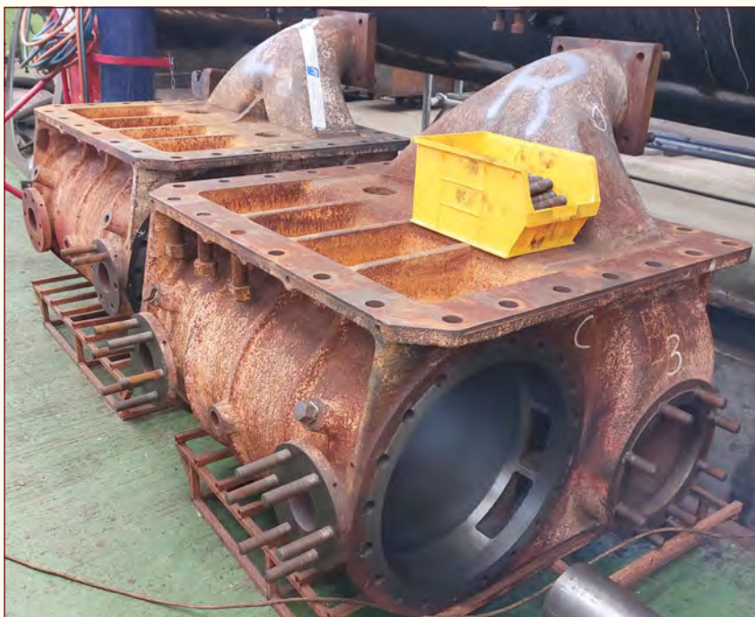
Above: One of 5551's Outside Cylinders being machined. The mountings for the Drain Cocks and Pressure Relief Valves can be clearly seen.
