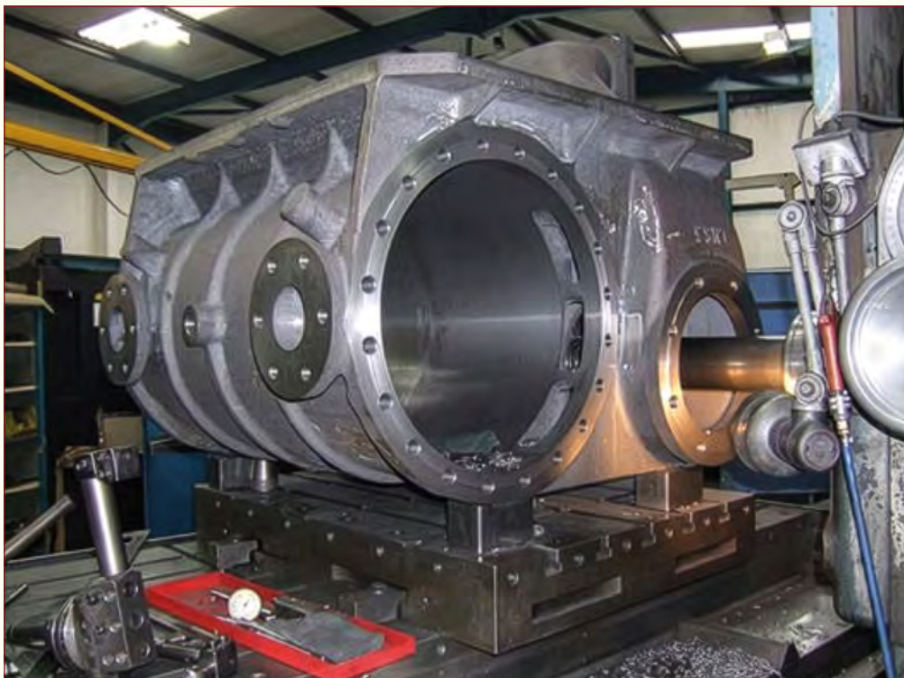
Above: One of 5551's Outside Cylinders being machined. The mountings for the Drain Cocks and Pressure Relief Valves can be clearly seen.
