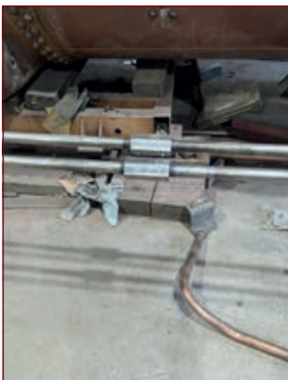
Remaining longitudinal stays fitted with buckles.
