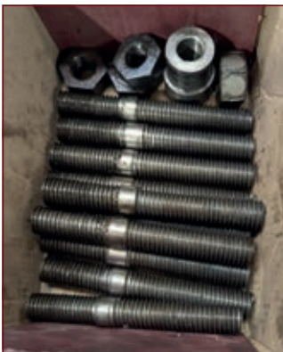
Internal dome studs for clamps of the copper pick-up pipes.
