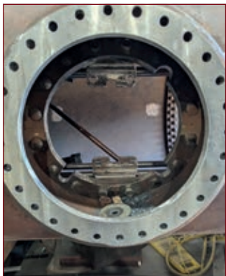
Recesses ground to allow better fitting of copper pick-up pipes.
