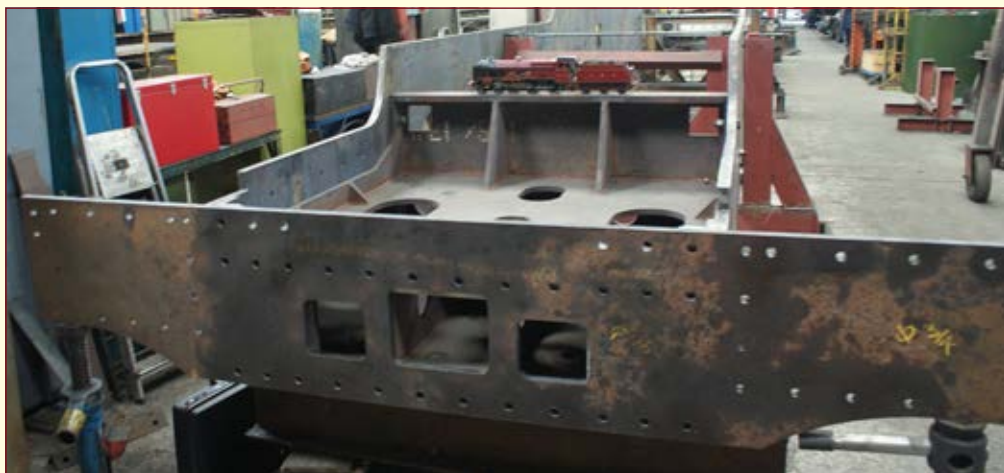
Above: Hind Beam and Drag Box positioned in the Frames at Llangollen. The authors Gauge 1 model of No. 5519 Lady Godiva is standing where the Boiler Slide will be mounted. Photo: Kevin West
