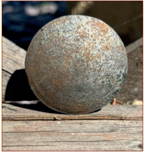
A rivet removed from 5551 during remedial work, shown at actual size with the domed head diameter being approximately 47mm.
