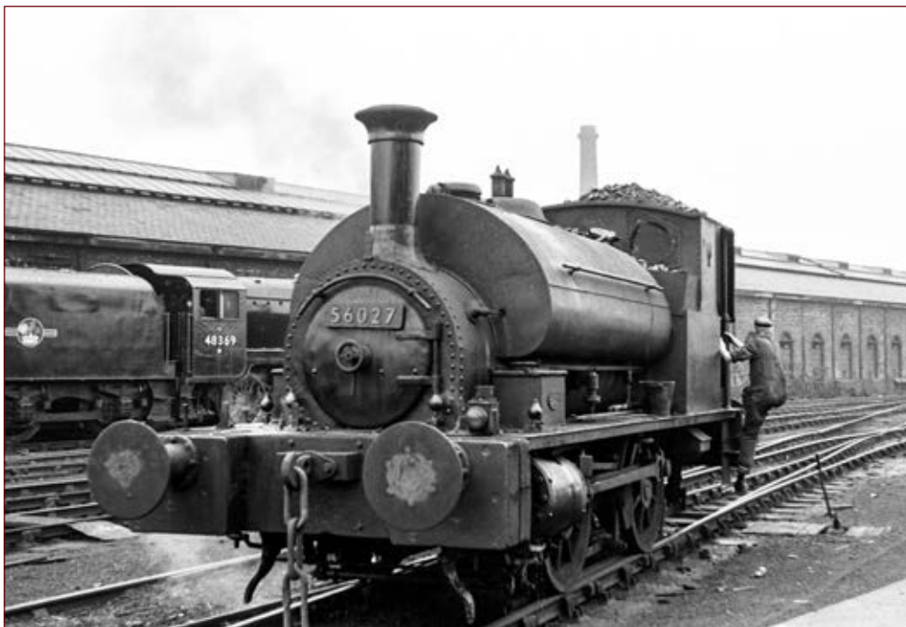
Built for the Caledonian Railway at St. Rollox Works, Glasgow in 1895, Class 264 0-4-0ST No. 56027 is seen working as the Crewe Works pilot. It was transferred to Crewe from Preston in January 1957 and worked there until withdrawal from service in October 1960. Note the coal stored on the cab roof. PHOTO: ALEC SWAIN © THE TRANSPORT TREASURY
