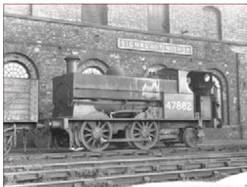
LNWR Class 317 0-4-2ST No. 47862 stands outside the Signal and Tin Shop (61 and 65 on works layout) shortly before withdrawal from service in 1956. Also known as Saddle Tank Shunter, Dock Tank or Bissel Tanks the class consisted of 20 square saddle-tanked steam locomotives built by the LNWR at Crewe Works between 1896 and 1901. They had a very short coupled wheelbase, with a trailing Bissel truck to carry weight. All passed to the LMS in 1923, who initially allocated them the numbers 6400-6419 in the passenger tank sequence. Only five had been renumbered before the numbers were changed to 7850-7869 in 1927, thus moving them into the goods and shunting tanks, changing their power classification from IP to 0F at the same time. Only two, 47862 and 47865, survived to enter British Railways service in 1948; 47865 was withdrawn in November 1953, and 47862 three years later. PHOTO: © THE TRANSPORT TREASURY
