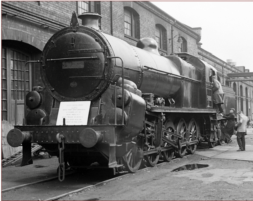
A final public viewing of No. 58100 at Deby on the occasion of the works open day. The engine had already been withdrawn, on 19th May 1956, reputedly due to a replacement boiler/firebox being required, both of which were of course non-standard and consequently with the cost not justified – note too the missing headlight already transferred to No. 92079. (The 3Fs were never fitted with a headlight as the driver was better placed to see the position of the rear of the train ahead due to the short length involved.) The board placed at the front described the principal dimensions along with the words, 'Formerly at Motive Power Depot Bromsgrove'. Even though it would never steam again the external condition is good, the engine having received lined BR black livery in April 1950 complete with the then BR crest. As with the Garratt types on BR, No. 58100 was never given a letter/number power classification. © TRANSPORT TREASURY
