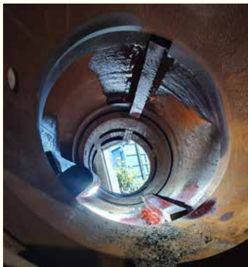
A view into the Valve Chest of one of the Outside Cylinders showing the new Port Bars in position. PHOTO BY PRCLT
