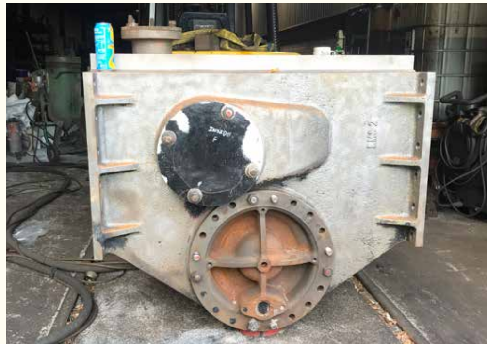
The middle cylinder after shotblasting. PHOTO: PETE SIKES
