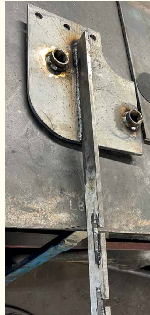
The new Front Buffer Beam following drilling all of the holes.
