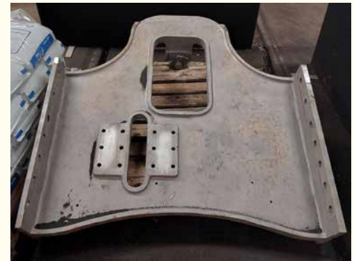
One of the Frame Stretchers following shot blasting.
