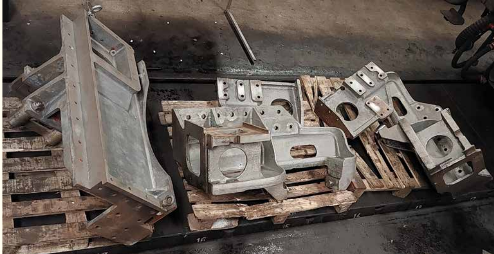
Chassis parts at West Shed ready for reassembly to the Main Frames following shot blasting and testing.
