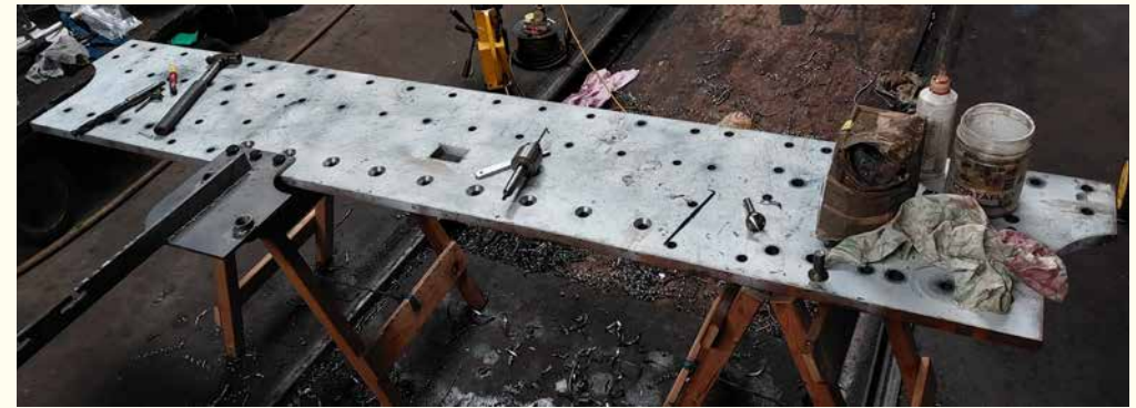
The new Front Buffer Beam following drilling all of the holes.
