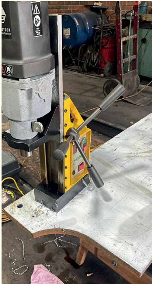
Marking out the Front Buffer Beam ahead of drilling (above) and the first hole is drilled (left). PHOTOS: PRCLT
