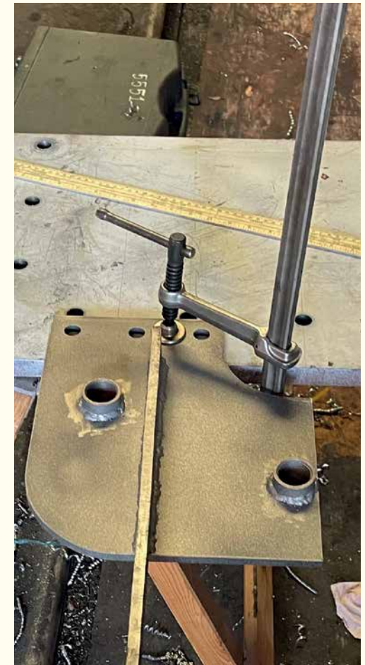
Left: The Air Brake Connection Mounting Plate and above showing where it is mounted on the front Buffer Beam. PHOTOS: PRCLT
