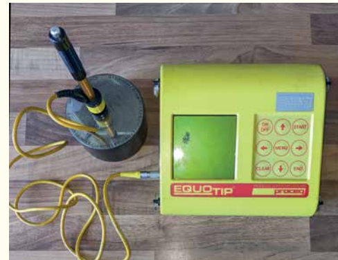
The equipment used for hardness testing.
