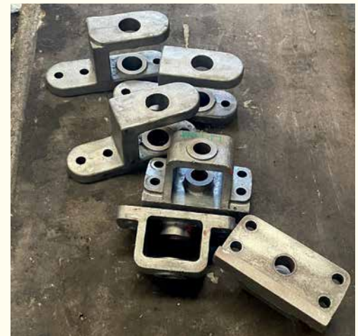
Spring and Brake Hangers following shot blasting.
