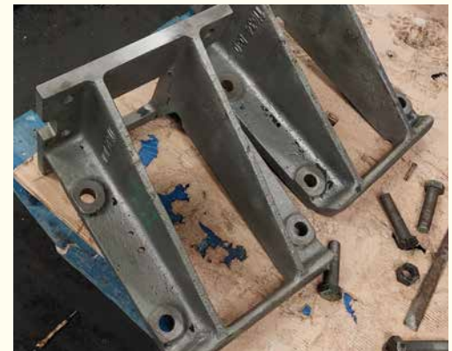
Valve Crosshead Brackets following shot blasting.
