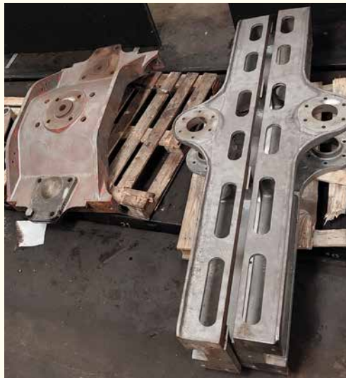
The Motion Girders and Bogie Centre Pin Casting following shot blasting.
