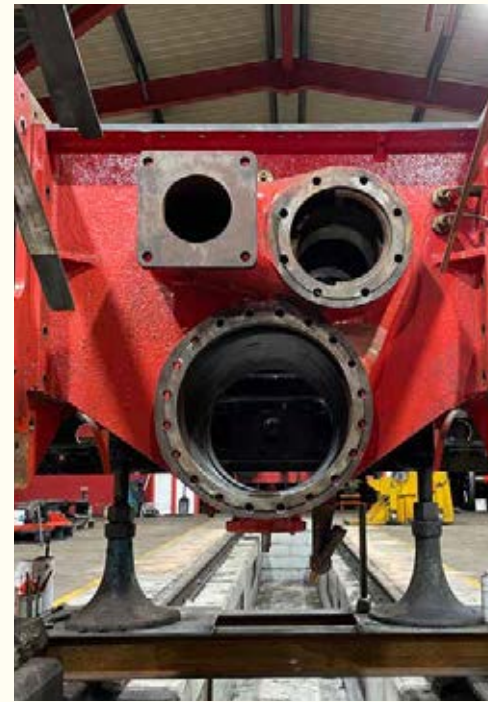
The chassis being prepared for removal of Inside Cylinder. PHOTO: ANDY COLLINSON
