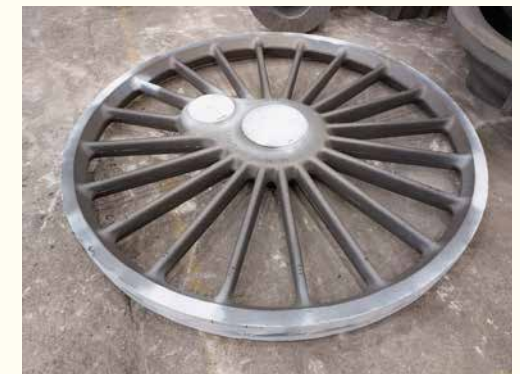
Driving Wheel casting for the B17 Spirit of Sandringham at William Cook's Cast Products.
