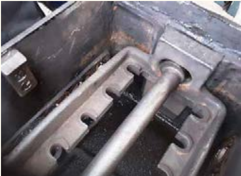
The Drive Cage on the Lubricator from 6203. The pump units have been removed to allow preparation of drawings. PHOTO: KEVIN WEST
