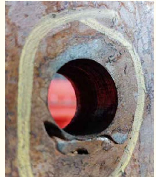
Poor welded repair on Frame Plate, Feb 2022. PHOTO: KEVIN WEST
