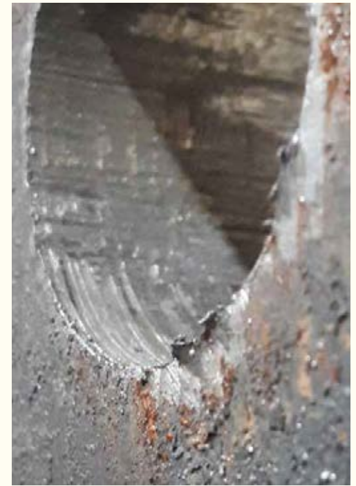
A close up of one of the Frame holes showing the burrs and the rough surface condition of the frame surface. PHOTO: KEVIN WEST
