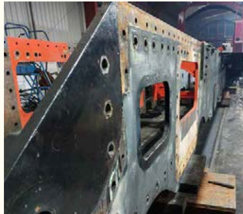
Inside and outside of frames prepared for repairs, February 2022. PHOTO: KEVIN WEST
