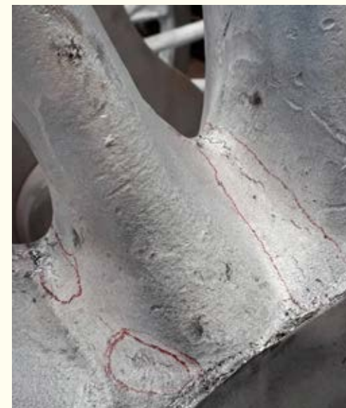
A view of one wheel with the surface cracks highlighted.
