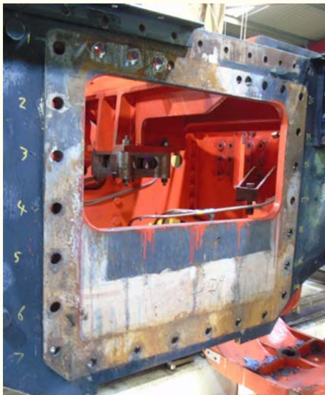
A view of the left-hand main frame following removal of the outside cylinder. The uneven surface where the cylinder sat can be seen.
