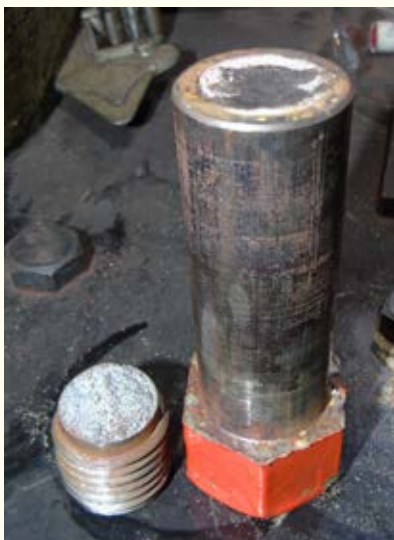
The previously-mentioned broken fitted bolt.
