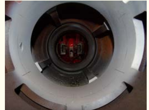
A view of the inside of the Inside Cylinder Valve Chest. The four guide bars can be seen running between the valve liners.
