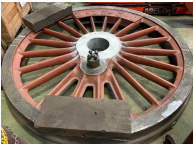
Left-hand Trailing Wheel following completion of welding repairs.
