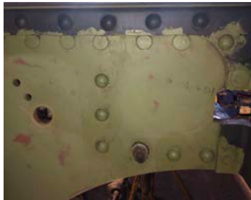
View of the rear left-hand main outer frame plate, showing the snap head and countersunk rivets holding the respective rear spacer box in place. The bolt still fitted is where the stay bolts go for the rear step, don't worry we didn't forget to fit one!
