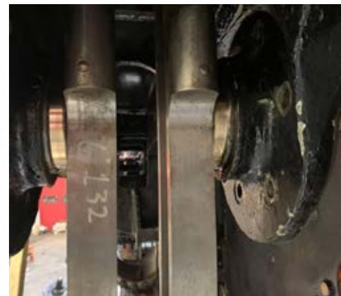
Expansion Link installed on the locomotive. PHOTO: PRCLT
