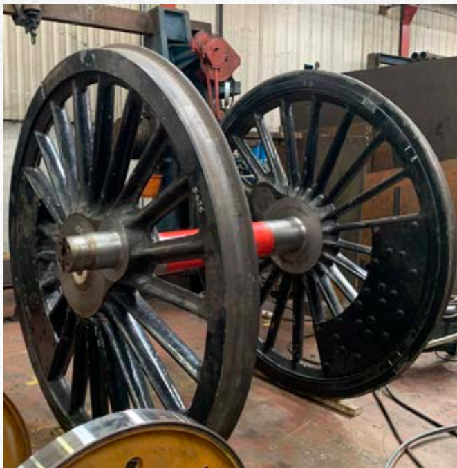
Centre Driving Wheel set following reassembly.
