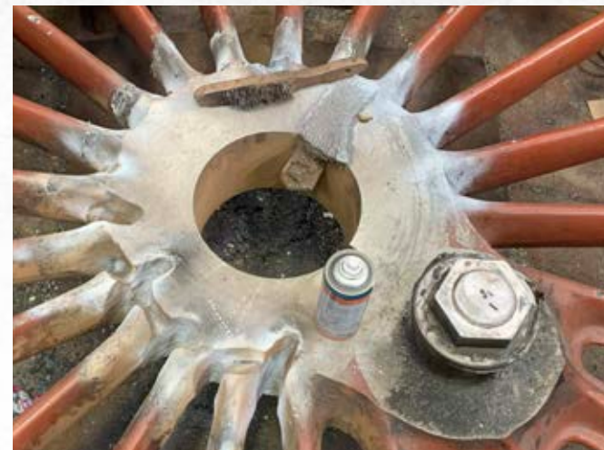
Right-hand Trailing Wheel showing where material has been removed to remove the cracks.
