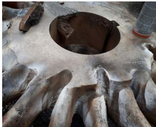
Closer view showing the extent of the cracks found.
