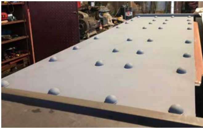
Rear drag-box top plate now riveted in place
