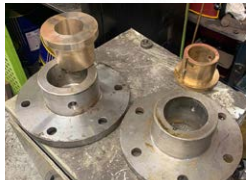
New Bronze Bearings ready to be installed in the mountings. PHOTO: PRCLT
