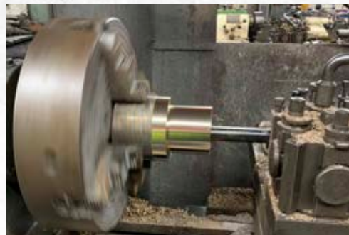
Expansion Link Bearing being machined. PHOTO: PRCLT
