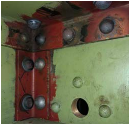
Internal shot of the inner section of rear dragbox, you can see the hole in the inside frames for the main brake hanger pin, the three smaller rivets hold the doubling plate for the pin in place on the inside frames.
