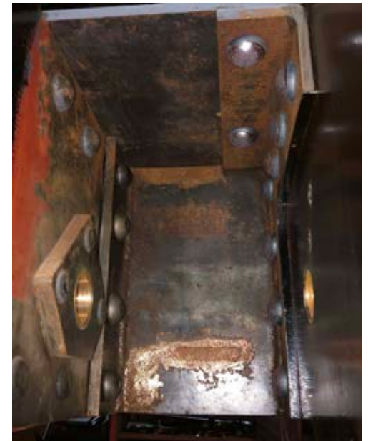
Shot showing the front of the left-hand rear spacer box. Inside frames on the left side of the shot with the brake pin doubling plate, the main outer frame plate is on the right-hand side in black.
