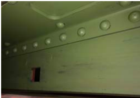
Internal view of the rear drag-box section, this will be covered up once the rear buffer beam is fitted.
