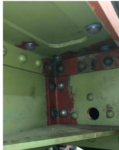
Another view of the inner section of rear dragbox. It becomes apparent when you see the number and position of rivets just how fiddly this has been, hence why we've triple checked everything before finally riveting it in place.
