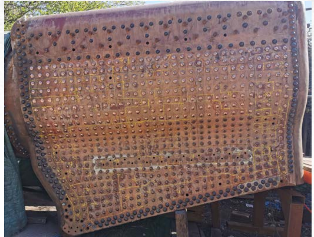
Above: View of the Firebox at HBSS showing installation of the side stays almost complete.
