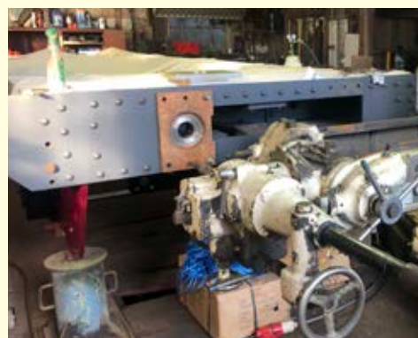
Reaming the holes prior to riveting the Intermediate Buffer Mounting in position.
