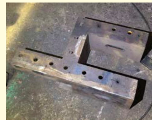
The left-hand Outer Rear Dragbox waiting to be installed between the main and inner frame plates.
