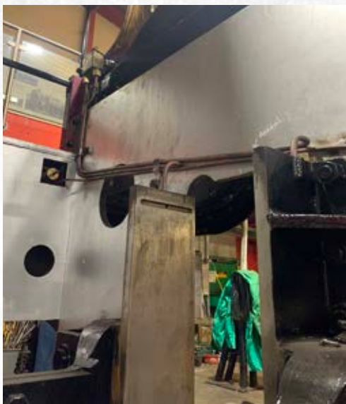
View of the left-hand Trailing Horn Guides. The guides are at the bottom of the picture with the pipework that supplies the oil to the horn faces clipped to the frames and leading up to the Oil Box. PHOTO: PRCLT
