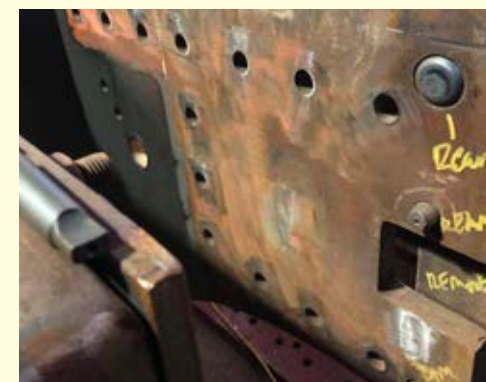
This view shows where the Outer Rear Dragbox is fitted between the Main and Inner frame plates.
