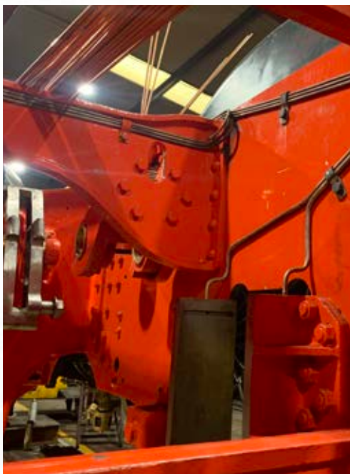
View of the right-hand Leading Horn Guides. The lubrication pipes to the horn faces can be seen fitted into the top of the Horn Guides. The fitting mounted to the frames at the top right is for the flexible oil feed into the axlebox. PHOTO: PRCLT
