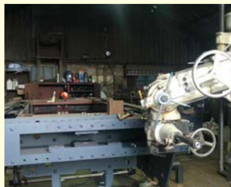
Drilling the Tender Front Buffer Beam for the Intermediate Buffer Mountings.
