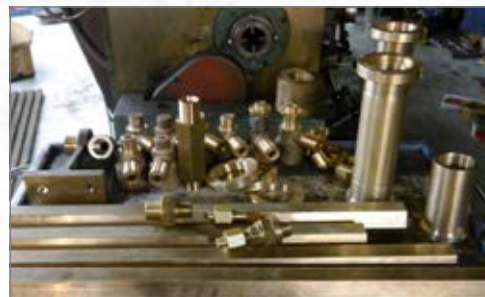
A selection of fittings and bushes after machining. PHOTO: ANDY COLLINSON
