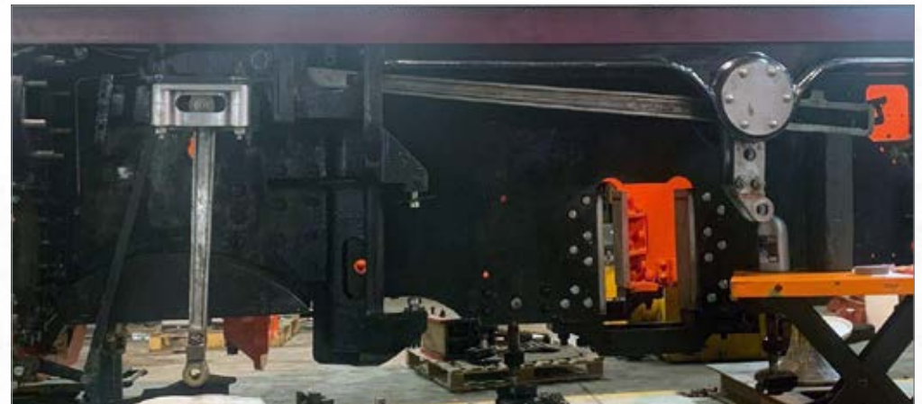
Below: The Radius Rod and Combination Lever mounted for clearance checks. PHOTO: PRCLT
