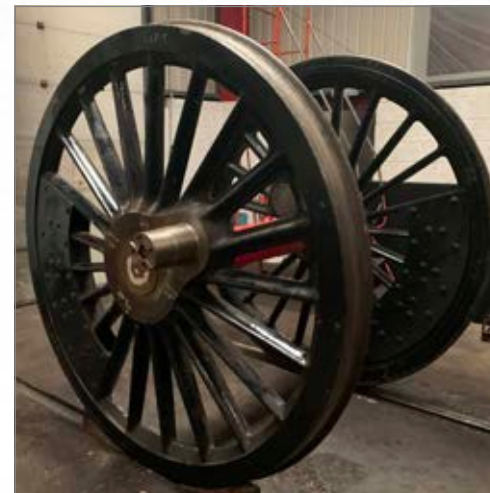
The Centre Driving Wheelset following delivery to West Shed. PHOTO: ANDY COLLINSON
