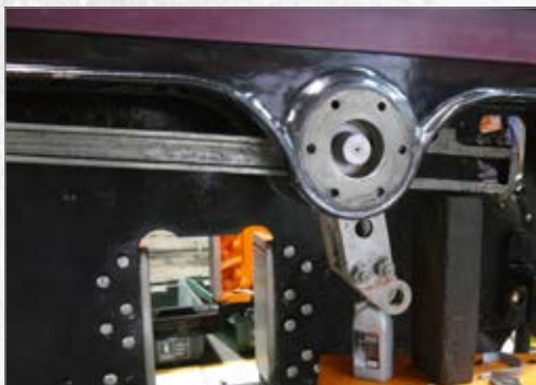
The left-hand Expansion Link undergoing checking. PHOTO: ANDY COLLINSON
