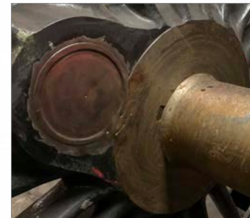
A view of the inside of the Centre Driving Wheel. This shows the Crank Pin at top left with the retaining ring formed over to lock it into the wheel. The axle is to the bottom right, covered in grease to protect the journal. At the joint between the axle and wheel can be seen the keyway, correctly positioned in line between the centre of the Axle and Crank Pin. This feature is the keyway incorrectly machined on three of the wheels. PHOTO: ANDY COLLINSON
