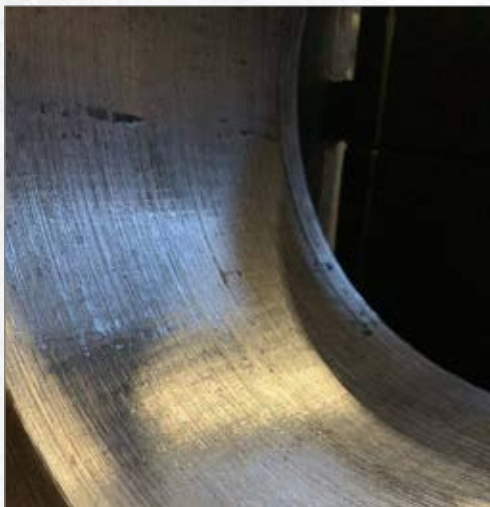
A view into the bore of one of the wheels following removal from the axle. One of the voids in the original weld can be seen at 9 o'clock. PHOTO: IAN RILEY & SONS
