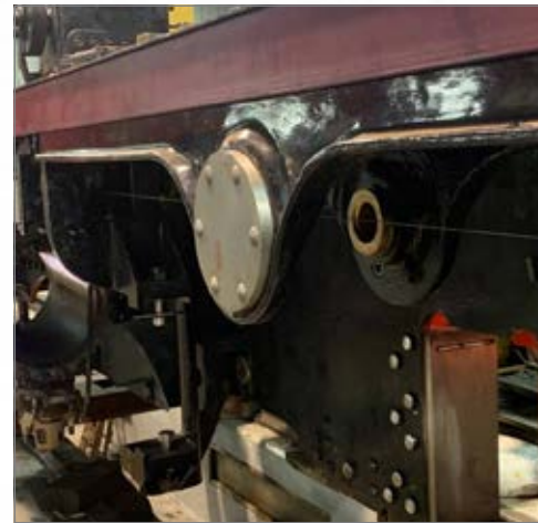
Above: Two views of the lining wire set up through the left-hand Valve Rod. BOTH PHOTOS: PRCLT.
