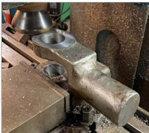
The Valve Rod Crosshead being machined. PHOTO: PRCLT
