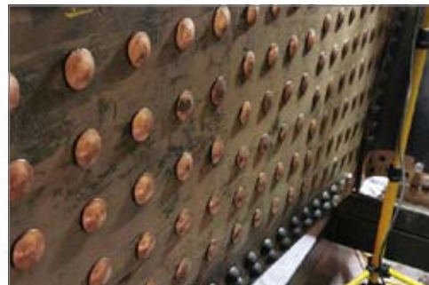
The Inner Firebox with the stays formed down. PHOTO: HBSS
