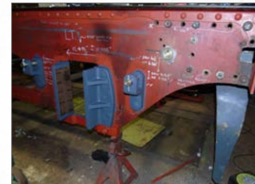
Left-hand rear end of the Tender chassis showing the Horn Guides and Spring Hanger Brackets in place. PHOTO: KEVIN WEST
