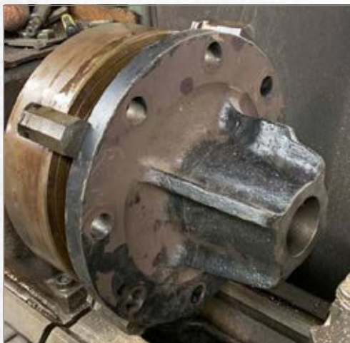
A Valve Chest Cover mounted in the lathe for some minor machining. PHOTO: PRCLT
