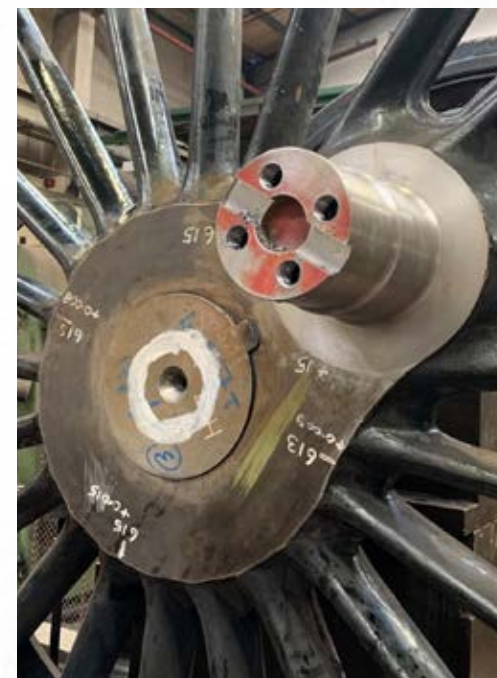
Above: The Centre Driving Axle ready for the new Crank Pins to be fitted. Below: After assembly. PHOTOS: RILEY & SONS (E) LTD.
