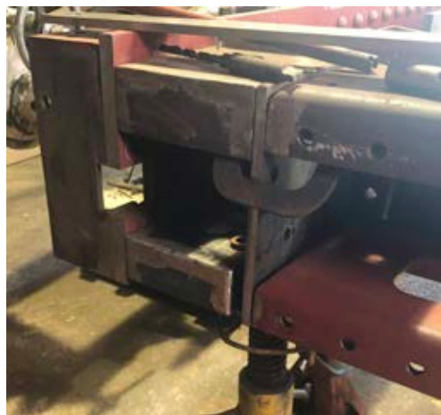
A view of the Rear Left Hand end of the Tender Chassis. From right to left we can see the upper and lower sections of the Centre Drag Box, the thinner Inner Frame plate, The Outer Drag Box, the thicker Outer Frame plate and finally the Outer Frame Angle. All this will be hidden from view when the Rear Buffer Beam is riveted into place.
