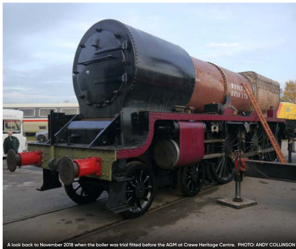
A look back to November 2018 when the boiler was trial fitted before the AGM at Crewe Heritage Centre. PHOTO: ANDY COLLINSON
