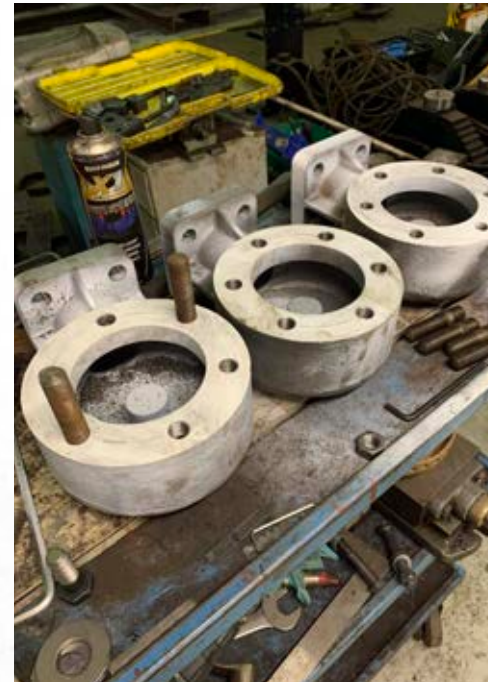
The three Snifting Valve Bodies following machining.
