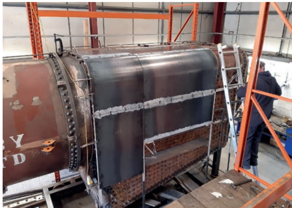
Firebox and Backplate Cladding in progress at HBSS. Photos: Heritage Boiler Steam Services
