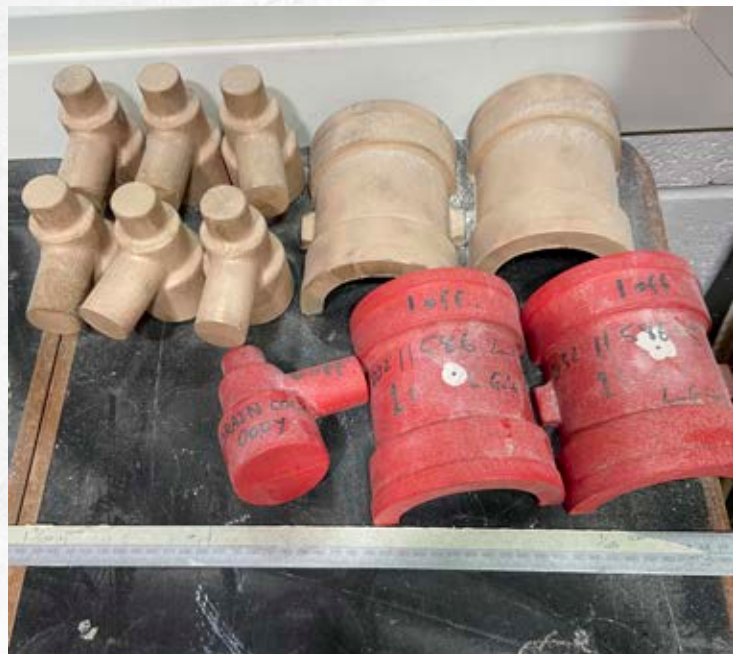
Drain Cock Castings and patterns. Photo: Premier Patterns
