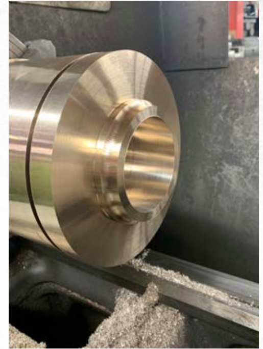
A Valve Head in process of turning.
