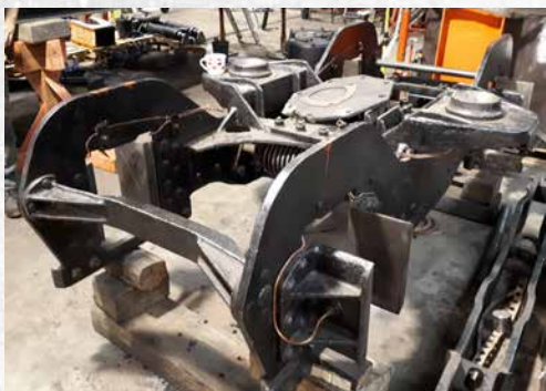
The Bogie frame from BR Class 4 No. 80097 in West Shed showing the shaped stretcher. 28th August 2019. Photo: Kevin West
