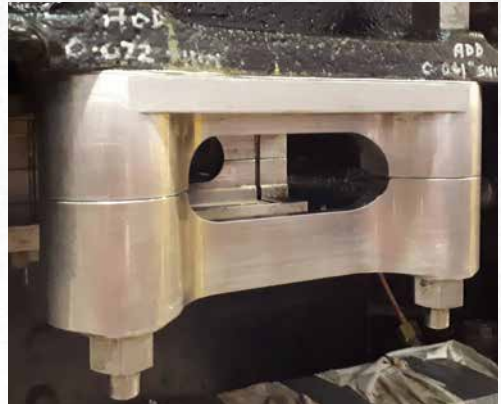
Right hand Valve Crosshead Guide after cleaning and polishing by PRCLT Volunteers. 28th August 2019. Photo: Kevin West
