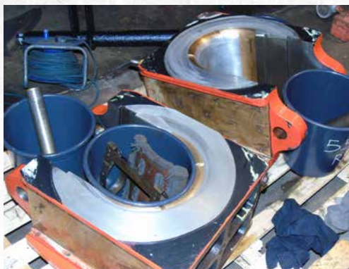
Axleboxes from 5551's trailing driving axle following removal at West Shed. Note all associated parts are stored in marked up buckets for safe keeping.
