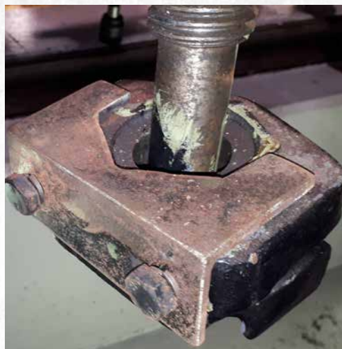
A Driving Axle Spring Clip showing the existing retaining bolts., 28th August 2019. Photo: Kevin West
