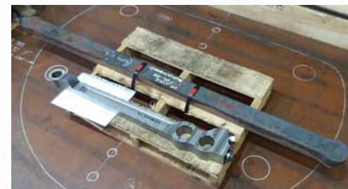
The flank cut blank for the Intermediate Reach Rod and the new Inside Combination Lever at CMS Cepercor.
