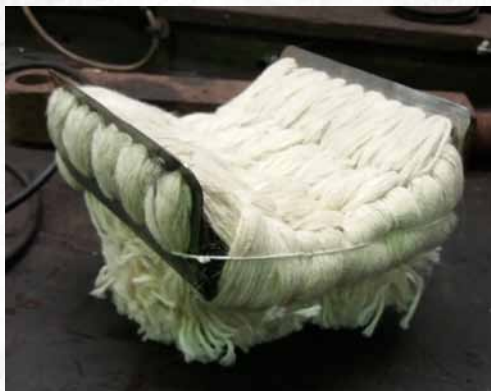
An Axlebox Bearing Lubrication pad.
