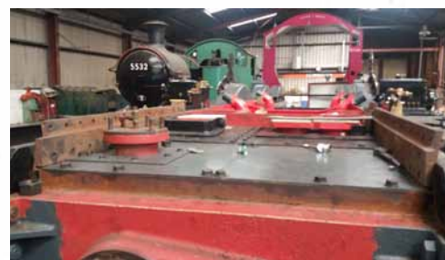
Two views of the Smokebox Floor Plates in position.
