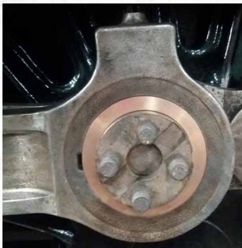
The left hand Connecting Rod Big End in position with a temporary bearing on 8th July.
