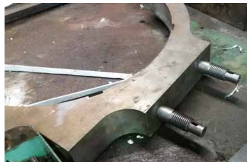
Eccentric Strap Front fitted with the fixing bolts for the Eccentric Rod.
