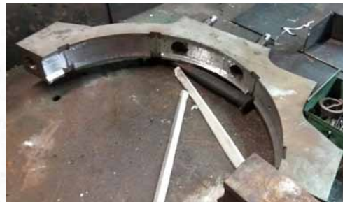
Eccentric Strap Front prepared for white metalling.
