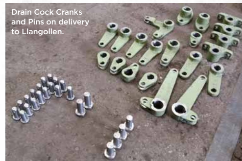
Drain Cock Gear parts on delivery to Llangollen.
