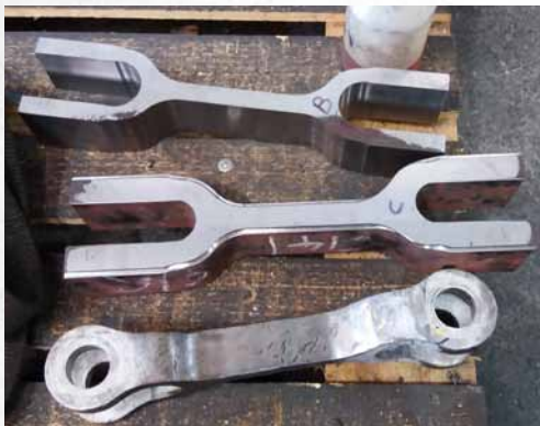
Union Links under manufacture at CMS Cepercor. The original at the bottom is from 45596 Bahamas .
