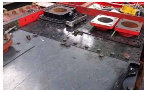
Two views of the Smokebox Floor Plates in position.
