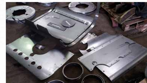
The Cylinder Clothing Sheets on arrival at Llangollen. The Main Sheets for the Outside Cylinders are in the top centre, with their end bands to the right. Below and left are the Outside Top Sheets with the Outside Bottom sheets to the right on top of the sheets for underside of the Inside Cylinder.
