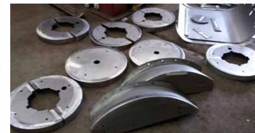
The Cylinder End Covers on arrival at Llangollen. The five covers split in half with the large cutout in the centre are for the hind end of each cylinder. There are five sets as three are in mild steel to be painted for normal use and two sets in stainless steel which will be burnished and polished for fitting to the Outside Cylinders when we finish the loco to an exhibition finish. There are also two sets for the front of the loco. In the foreground are the two splashers for behind the Outside Cylinders.
