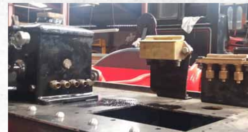
Oil Boxes mounted on the right platform.
