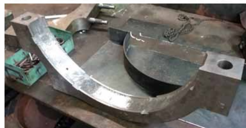
Eccentric Strap Rear prepared for white metalling.
