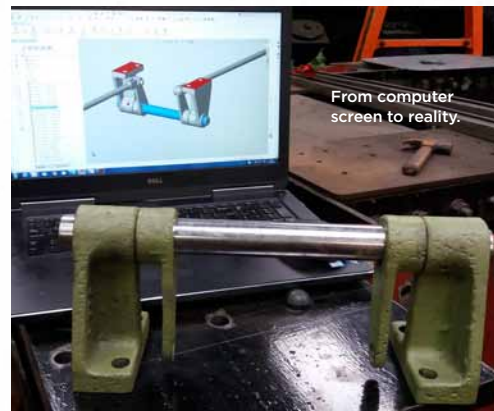
Eccentric Strap Front fitted with the fixing bolts for the Eccentric Rod.
