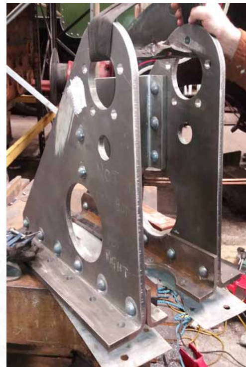
The Brake Cross Shaft Bracket after riveting.
