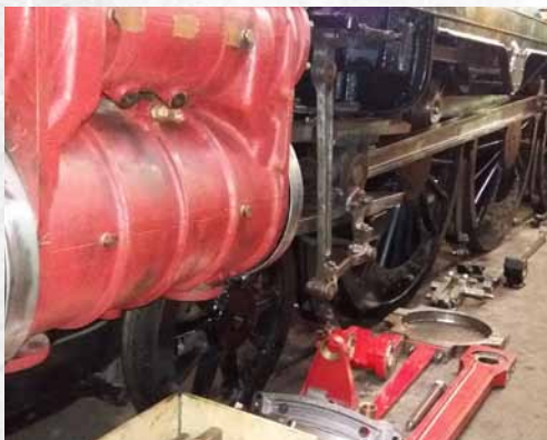
The Unknown Warrior, with most of the left hand valve gear fitted. 8th July 2017.
