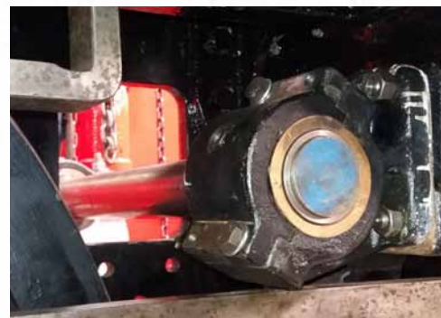
Two views of the Main Reverser Shaft Outer Trunnions in position. The Inner Trunnions can be seen through the square hole in the Frame Plate, with the three mounting holes below.
