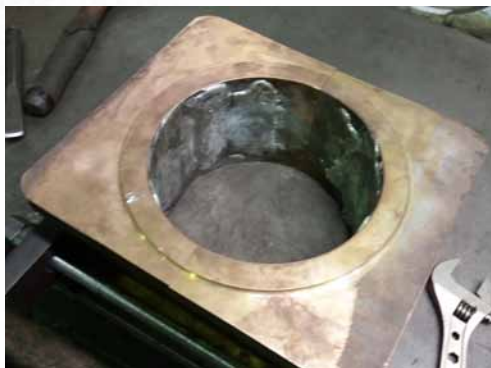
Inside Big End Brasses undergoing white metalling.
