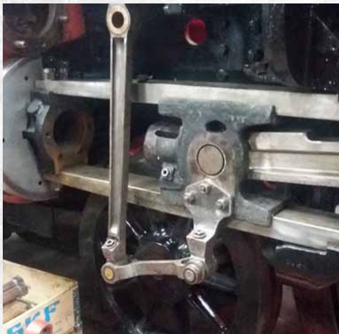
Left Hand Valve Gear as displayed at Members' Day 8th July 2017. Most of the parts seen here are refurbished Jubilee class parts.
