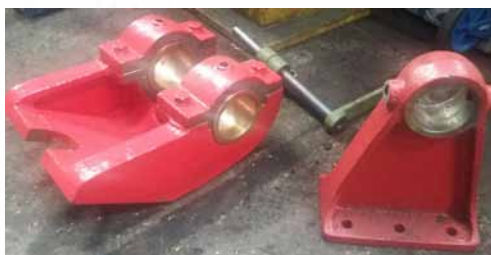
The Inside Reverser Shaft Bracket and one of the Inside Expansion Link Trunnions.
