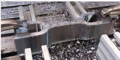
A Union Link undergoing machining.
