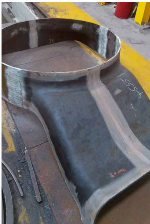
The Throatplate following completion of welding at LNWR, Crewe. Both photos: Jordan Leeds
