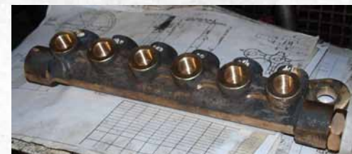
The Atomiser body being machined at Tyseley Locomotive Works.
