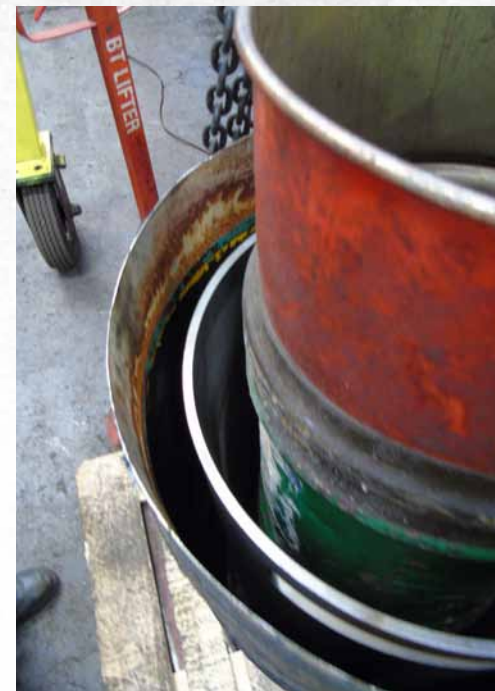
A liner in the nitrogen bath before being filled with nitrogen. The inner drum is there to reduce the amount of liquid nitrogen used.
