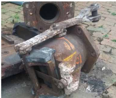
The Regulator from 8F No. 48518 which is to be used in The Unknown Warrior. Behind is the 8F J Pipe which is unfortunately not suitable for use. On the floor is a Horn Guide casting from Great Eastern Railway 0-4-OST No.209.
