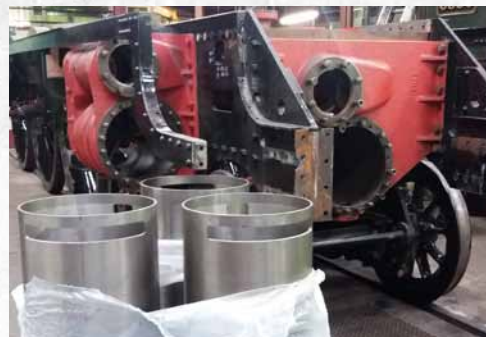
The Front Buffer Beam has been removed to allow easy access to the cylinders. The Liners can be seen in the foreground.
