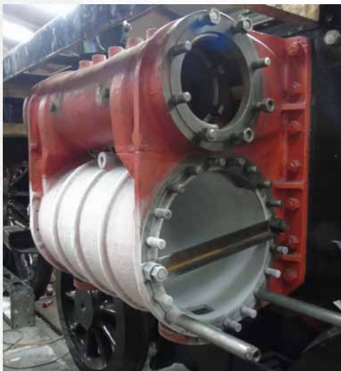
The right hand Cylinder following fitting the liner. The cylinder casting has frosted due to the freezing of the liner.
