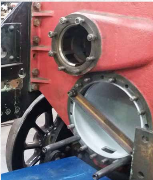
The Inside Cylinder following fitting of the liner. The retaining bars are fitted to stop the liner creeping in the bore as it warms up.
