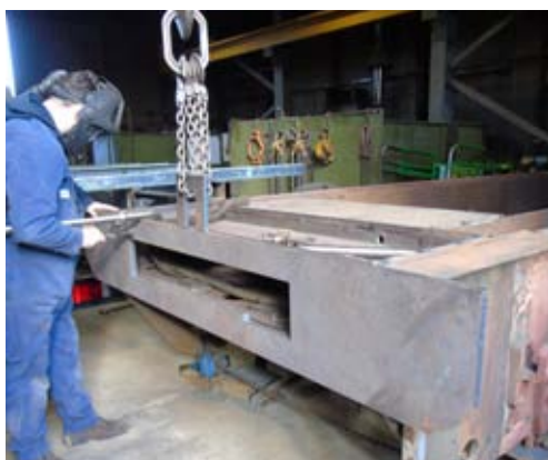
▲ Mathew Walker clamps the new Front Buffer Beam into place.
