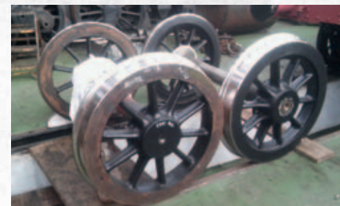
▲ The Bogie Wheelset after tyre turning. PHOTO: KEVIN WEST
