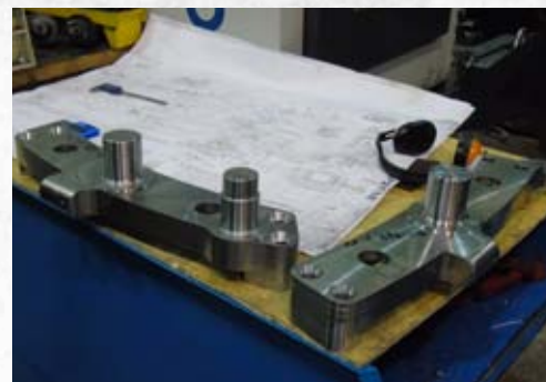
The Expansion Links after machining. PHOTO: KEVIN WEST
