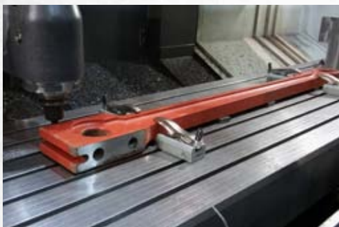
▲ Inside Connecting Rod undergoing machining. PHOTO: KEVIN WEST
