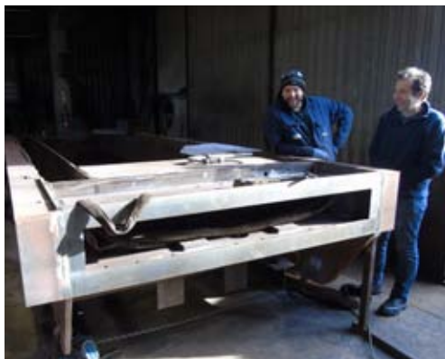
▲ Mathew Walker and Andrew Kennedy from Oakwood Visuals inspect the new Front Drag Box in place at Rowlescourt Engineering.
