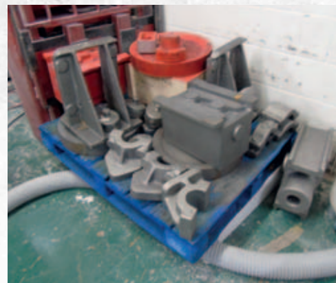
▲ A selection of castings at Premier Patterns: Valve Crosshead Bracket, Sandbox Lids, Reverser Shaft Trunnions, Lubricator Body and Inside Crosshead. PHOTO: KEVIN WEST
