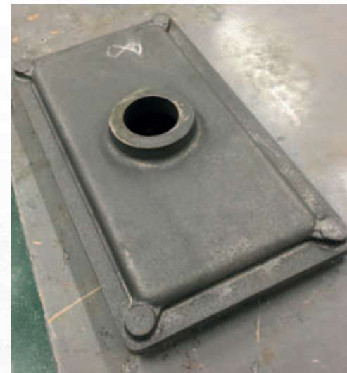
▲ Lubricator Lid Casting. PHOTO: KEVIN WEST
