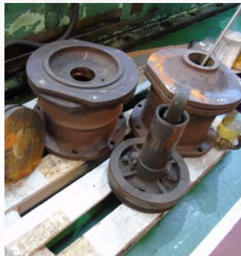
Brake Cylinders under overhaul at Harco Engineering. PHOTO: KEVIN WEST
