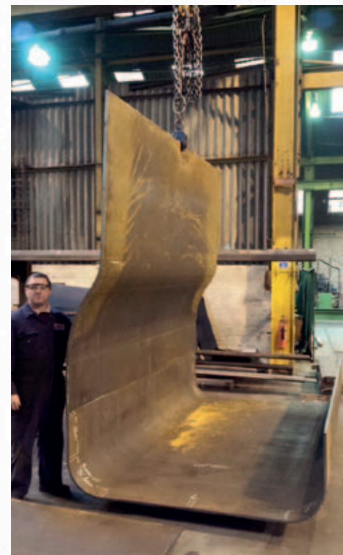
▲ Outer Firebox Wrapper sheets during forming at Deepdale Engineering. PHOTO: OAKWOOD VISUALS
