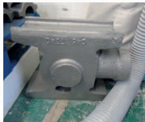
▲ Crosshead casting. PHOTO: KEVIN WEST
