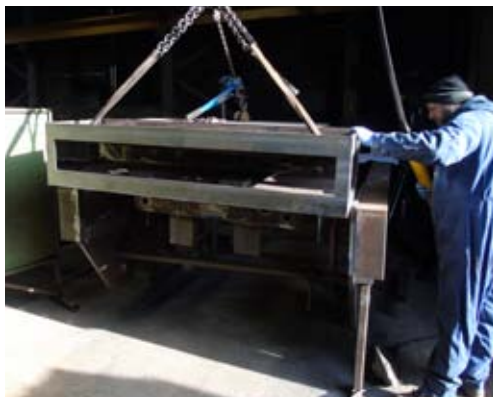
▲ Mathew Walker guides the new Front Drag Box into place on the restored Tender Frames at Rowlescourt Engineering on 11th February.
