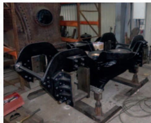
▲ The Bogie Frame under assembly at Tyseley. PHOTO: DAVID BRADSHAW
