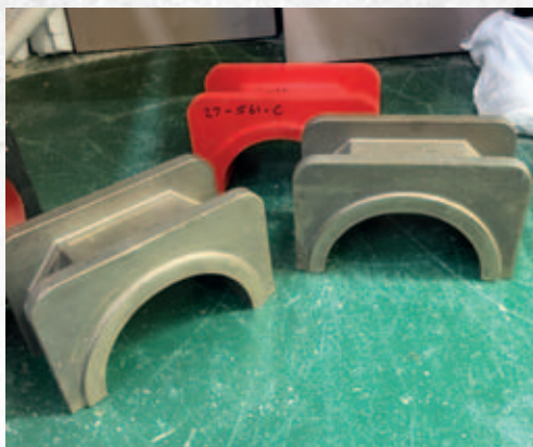
▲ Big End Bearing casting. PHOTO: PREMIER PATTERNS
