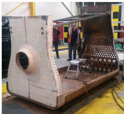
▲ Inner Firebox assembly underway at LNWR Crewe. PHOTO: GAVIN SHELL
