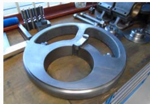
The Eccentric for the inside Valve Gear after machining at Harco Engineering. PHOTO: KEVIN WEST
