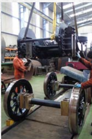
◀ The completed Bogie Frame being lowered onto its wheelsets at Tyseley.
