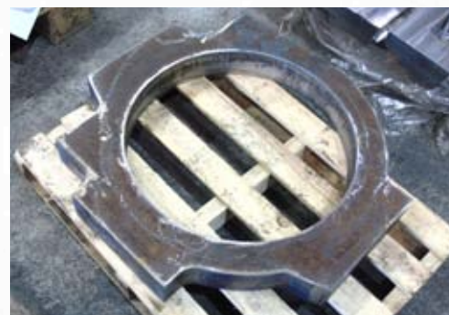
The flame cut blank for the Eccentric Sheaf Halves at Rowlescourt Engineering on 11th Feb. PHOTO: KEVIN WEST
