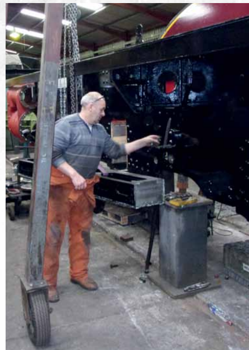
Just before The Warrior went to press in late July these images were taken showing the latest progress on the engine. The photos above show Chris Collins trial fitting the motion girder to the frames. Below are views of the inside of the frames and the right hand cylinder with the motion bracket fitted.
