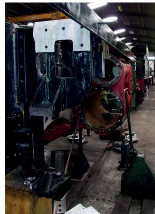
Just before The Warrior went to press in late July these images were taken showing the latest progress on the engine. The photos above show Chris Collins trial fitting the motion girder to the frames. Below are views of the inside of the frames and the right hand cylinder with the motion bracket fitted.
