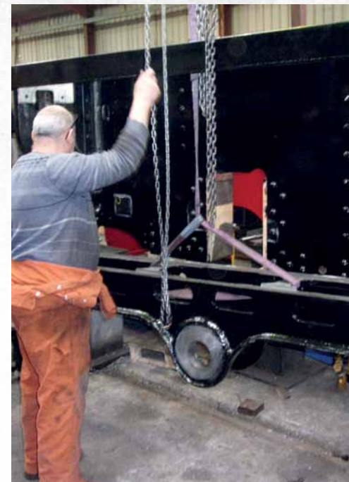
Just before The Warrior went to press in late July these images were taken showing the latest progress on the engine. The photos above show Chris Collins trial fitting the motion girder to the frames. Below are views of the inside of the frames and the right hand cylinder with the motion bracket fitted.
