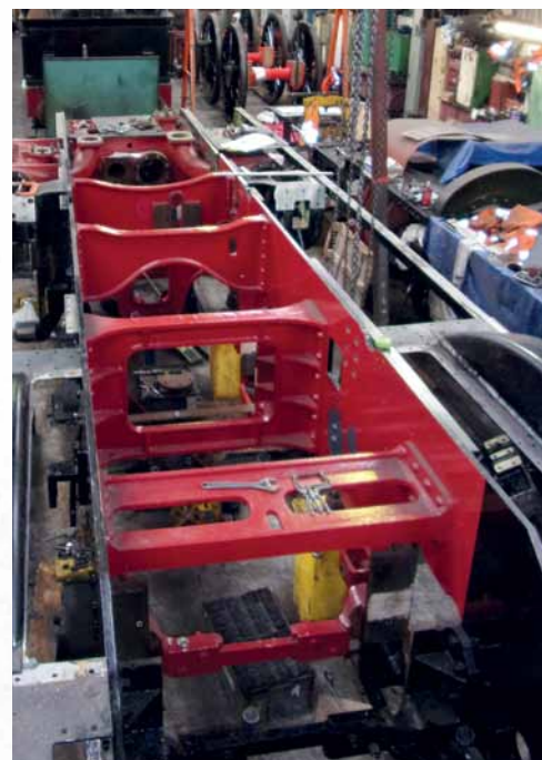
Just before The Warrior went to press in late July these images were taken showing the latest progress on the engine. The photos above show Chris Collins trial fitting the motion girder to the frames. Below are views of the inside of the frames and the right hand cylinder with the motion bracket fitted.
