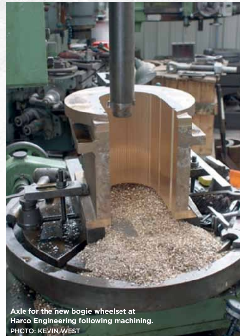
Bogie wheel being machined at Harco Engineering. PHOTO: HARCO ENGINEERING
