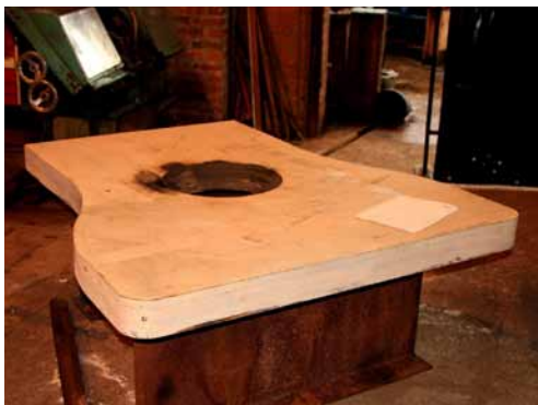
▲ Wooden former made for the inner firebox backplate. PHOTO BY KEITH LANGSTON
