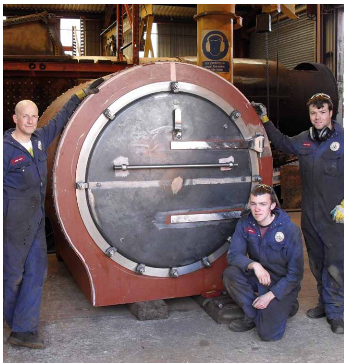
Smokebox for 'The Unknown Warrior' is seen after completion at LNWR Crewe on 31st May with LNWR Heritage employees John Liddell, Dan Lovatt and Bradley Walsh. Photo by Oakwood Visuals
