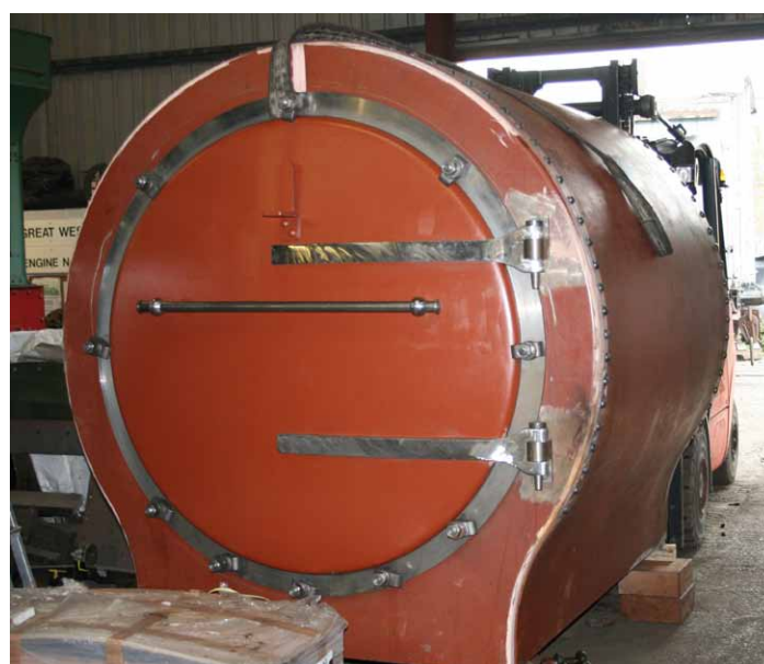
Above: Completed smokebox before painting being delivered to the Llangollen Railway Works on 5th June 2013. Photo by John Bennett.
