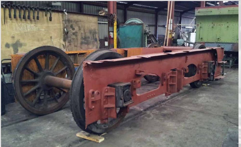
The frames from the Fowler tender purchased from the ELR are seen at the Llangollen Railway Works during April. Photo by Andrew Laws
