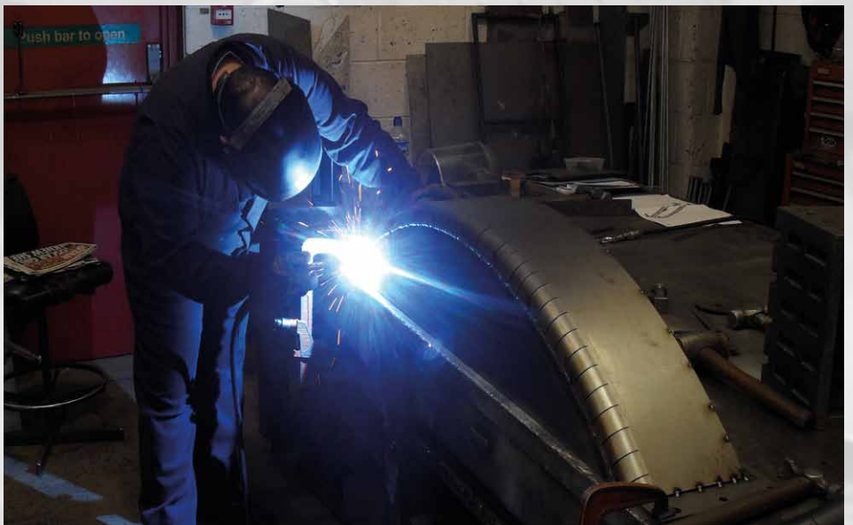
The six driving wheel splashers have now been made for 'The Unknown Warrior'. Photo by Oakwood Visuals
