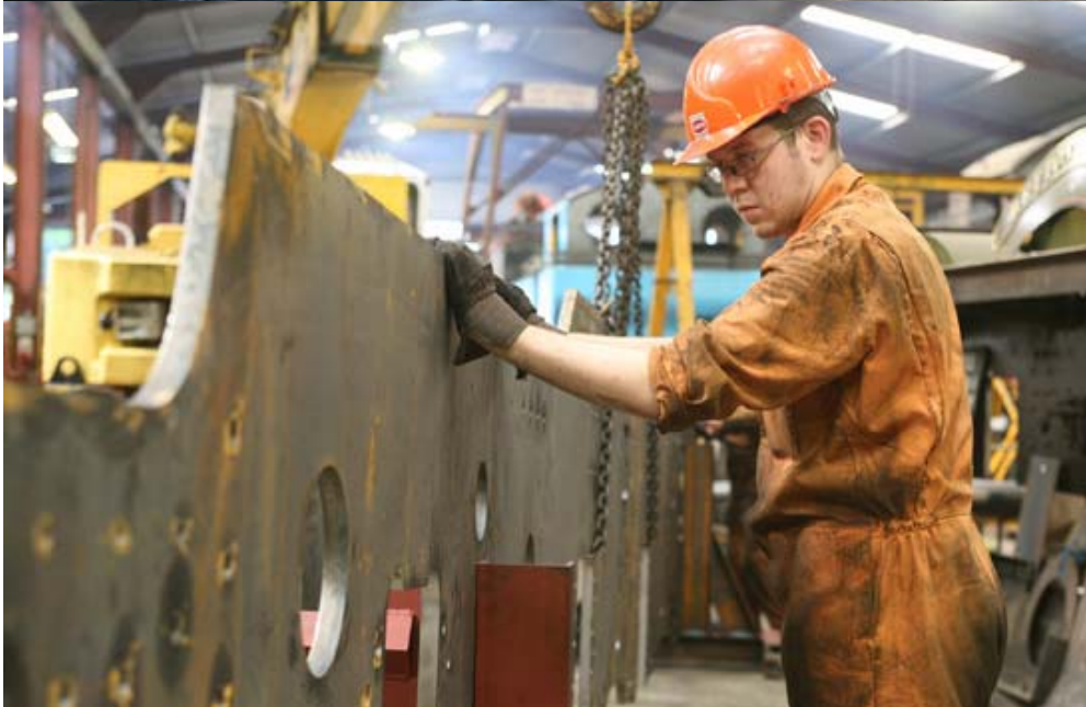
The two frame plates are held in specially made steel stands until the stretchers that will join the two plates together arrive.
