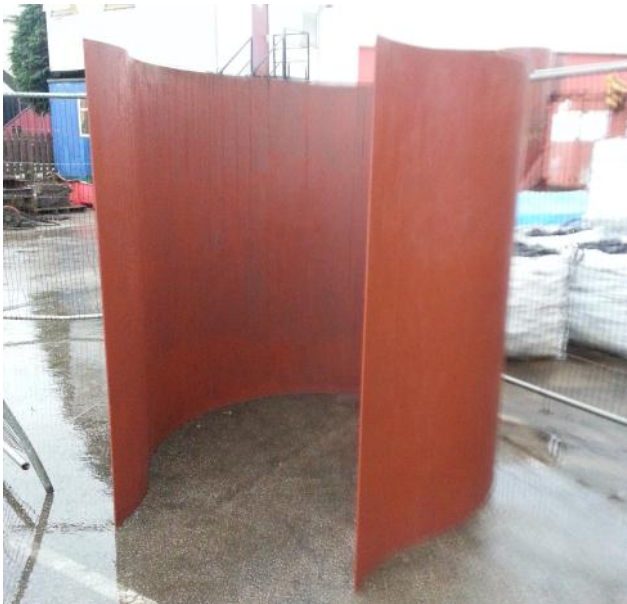
Smokebox wrapper and tube plate for the boiler for 'The Unknown Warrior' are seen on November 9th at LNWR Crewe. Photos by Gavin Shell.
